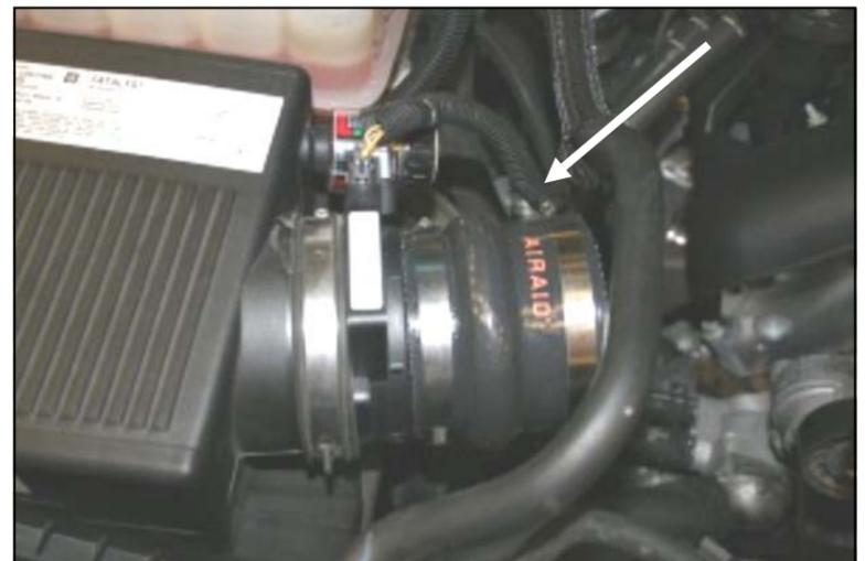
4. Install the hump hose (#3) and two #60 hose clamps (#5) on the Mass Air Flow sensor as shown. Leave the clamps loose for now.
