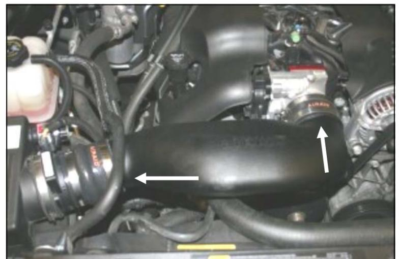
6. Install the **Modular Intake Tube** (#2) into the hump hose first, and then into the throttle body. Adjust for fit, and tighten all four hose clamps. Re-insert the plastic piece from step #3 into the hole on the bottom of the MIT.
