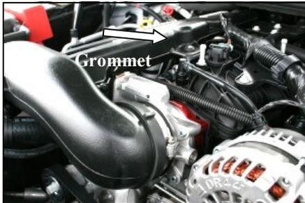
9. Re-install the intake tube using caution to center the intake tube hole over the previously installed grommet. Some adjustment may be required to seat the grommet correctly back into the intake tube. Tighten the hose clamps on the tube. Re-connect the breather tube. Re-install the plastic holder from step #1. Re-install the beauty cover. **Re-connect the negative battery cable!**
