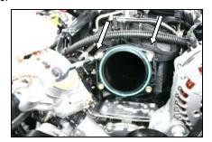
**4.** With a 4mm socket, remove the two studs that held the throttle body to the intake manifold.
