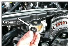
7. Remove the factory grommet from the intake tube.
