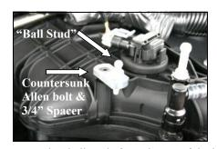
**6.** Remove the "ball stud" from the top of the intake manifold, insert the countersunk Allen bolt (#6) thru the countersunk hole in the provided 3/4" spacer plate (#5). Thread the countersunk bolt into the hole where you removed the "ball stud", face the spacer towards the front of the vehicle, and tighten the countersunk Allen bolt. Next thread the "ball stud" into the forward hole in the 3/4" spacer and tighten.
