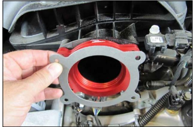
3. Install the Poweraid Spacer into the intake manifold with the supplied gasket on the throttlebody side, as shown. \*Note: Poweraid spacer must be installed with bore protruding into intake manifold away from throttle body. Incorrect installation will hinder performance. Reference picture below for spacer orientation
