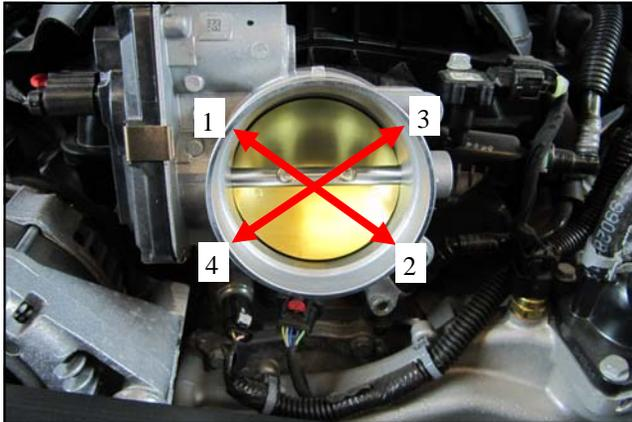
4. Insert the provided bolts with washers through the throttlebody, gasket, and Poweraid Spacer and tighten them in an "X" Pattern.
