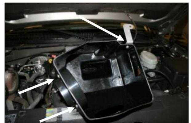
6. Install the filter adapter (#4) into the Cool Air Box (#3) as shown using three 1/4" Button head bolts (#8) and three 1/4" flat washers (#11). Next, fasten the bracket (#15) to the front of the CAB as shown using one 1/4-20 hex bolt (#9) two flat washers (#10), and one 1/4" Nylock nut. Refer to the drawing above for reference.
