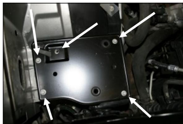
5. Using a 10mm socket, remove the bolts that secure the factory air filter housing platform and remove it from the vehicle.
