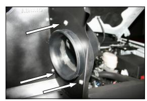
**6.** Install the Airaid intake tube (#4) into the Cool Air Dam using the three 1/4"-20x1/2" button head bolts (#6), and washers (#7) as shown.
