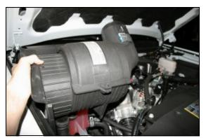
3. Slide the flexible intake tube off of the factory airbox and then rock the airbox back and forth to free it from the mounting grommets, then lift it straight up and remove it from the vehicle.
