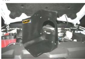
**5.** Assemble the two Cool Air Dam panels (#2) and (#3) as shown, using the five 6-32 screws (#10), washers (#11), and nuts (#12). Apply the Airaid Foil Decal onto the Panel as shown.
