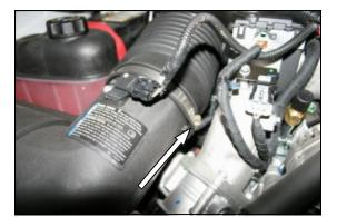
1. <u>Disconnect the negative battery cable.</u> Using a 5/16" socket or flat screwdriver, loosen the hose clamp that holds the factory airbox to the flexible intake tube.
