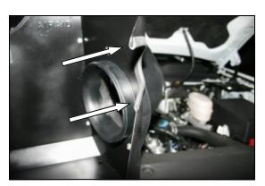
7. Install the supplied rubber trim (#13) onto the Cool Air Dam as shown.
