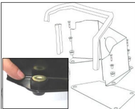
**4.** Assemble the Airaid Cool Air Dam panels (#2, #3) using the factory rubber grommets and inserts as shown.
