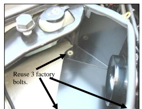
**6.** Install the Airaid Cool Air Dam over the three factory mounting points, and fasten with the factory bolts saved in step #2.
