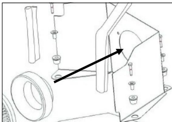
**5.** Install the filter adapter (#4) into the Airaid Cool Air Dam using three 1/4-20x 5/8" bolts (#6), and 1/4" flat washers (#7).
