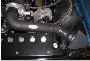
14. Connect the performance airbox assembly to your throttle body or carburetor by using any combination of Airaid's UBI components.
