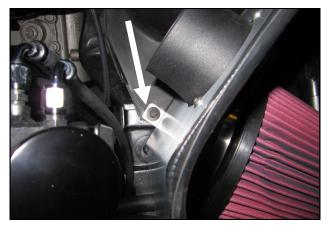
7. Align the Aid Dam tab with the factory bolt hole from step #3 and secure it by reusing the factory bolt.
