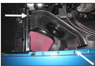
**6.** Carefully install Air Dam assembly in to the inner fender area. **Note-**The outermost edges will be underneath the core support and the fender when installed
