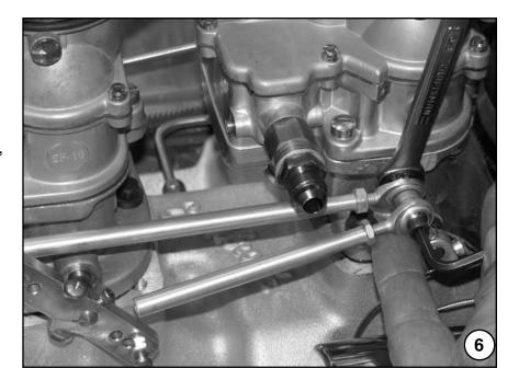
5) Connect forward rod end of slide link to the throttle arm of the center carb. Adjust slider link so that all 3 carbs reach WOT at the same time. Picture 7.
