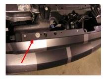
10) Lift the top of the bumper up and over the tabs. Then, slide the whole bumper cover forward and off of the vehicle.
