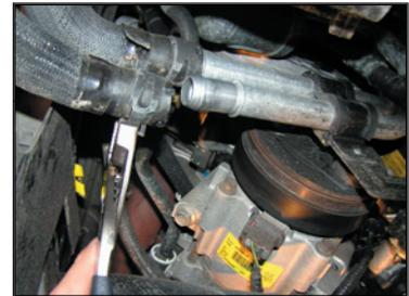
12. Disconnect the wiring harness from the pass. side driving light.
