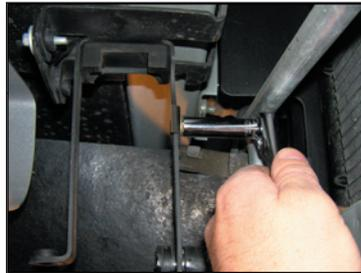
9. Remove the heat exchanger asm. from the vehicle.
