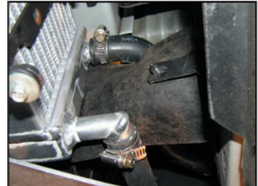
23. Install the black wire tie to prevent the lower hose from rubbing on the splash shield.
