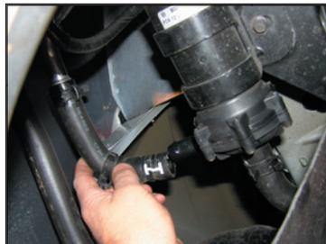
11. Disconnect the heat exchanger outlet hose from the engine. It is connected to a steel line just below the A/C compressor. You will disconnect the lower of the two hoses.
