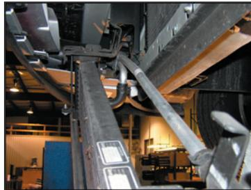
6. Disconnect the lower hose to drain the coolant.
