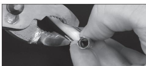
7. Place the open end of the terminal facing the "W" in the crimper tool.
