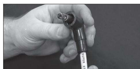
12. For HEI style boots: lightly lubricate the terminal with dielectric grease and slide the wire into the HEI boot.
