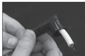
3. Utilizing the 7mm or 8mm holes on the ACCEL Wire Crimper, slide the wire through the hole with the end flush.
