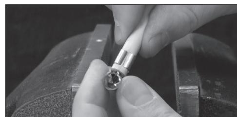
11. For points style terminals: slide the boot onto the terminal.
