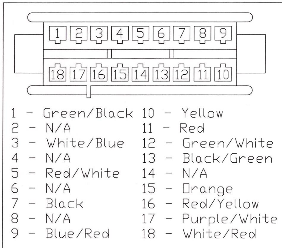
Figure 7-38 1973 - 1974 Cluster Pigtail Pinout
