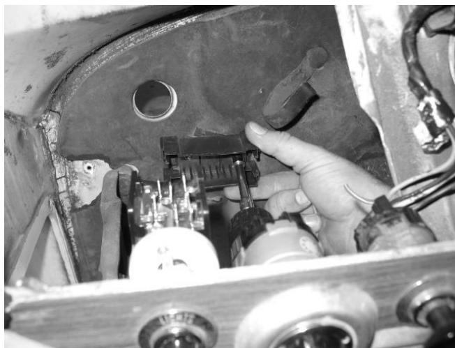
Figure 6-2 Fuse Block Base Position '67-'72
