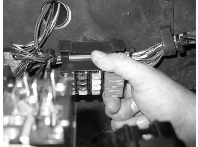
Figure 6-5 Snapping Fuse Block into Base
