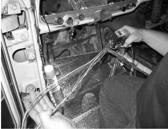
Figure 6-4 Routing Fuse Block to Base
