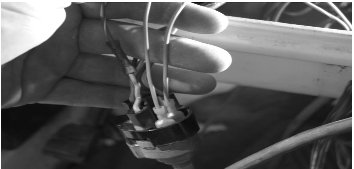
Figure 7-21 Wiper Switch w/wires connected
