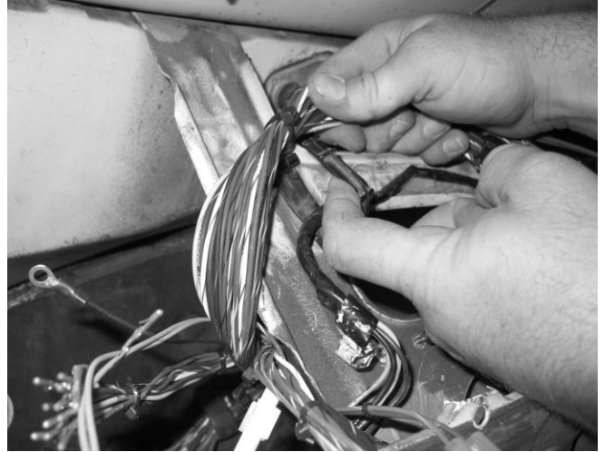
Figure 6-8 Steering Column Harness Clips
