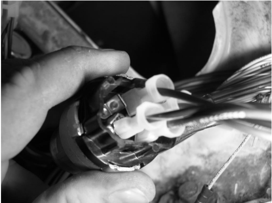
Figure 7-17 Ignition Switch Connections
