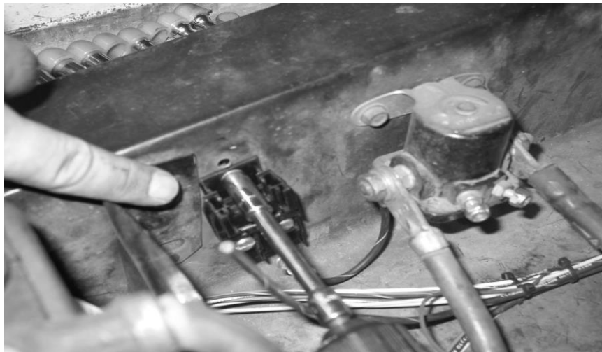
Figure 7-5 Installing the Maxi Fuse Holder '67-'72 Models
