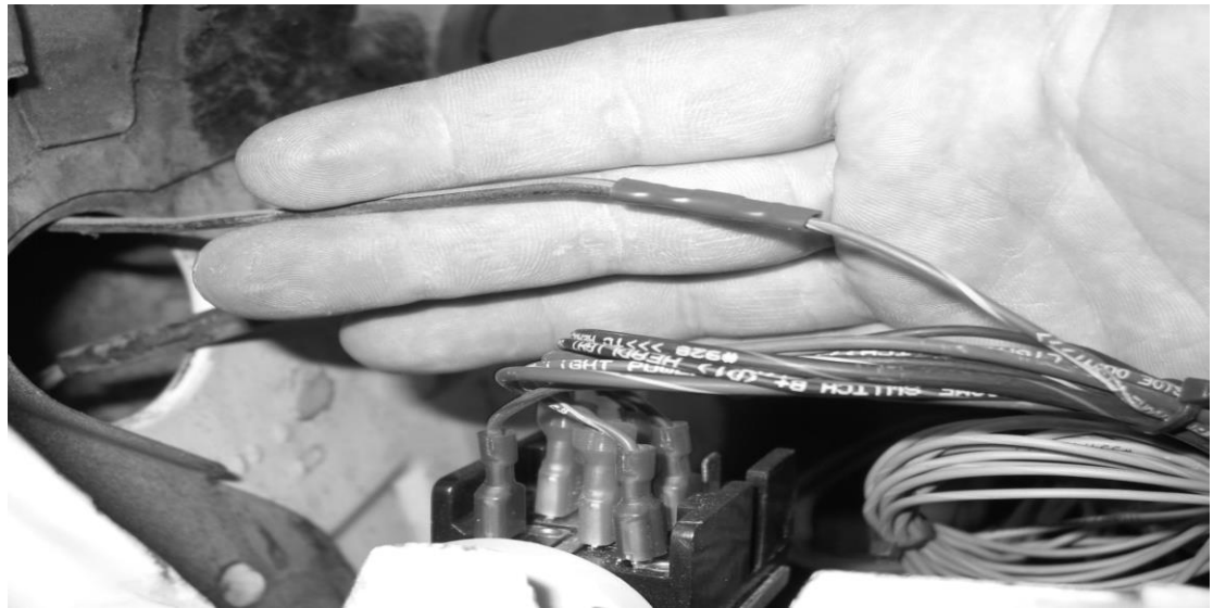
Figure 7-27 Dome Light Power Wire (All Models)
