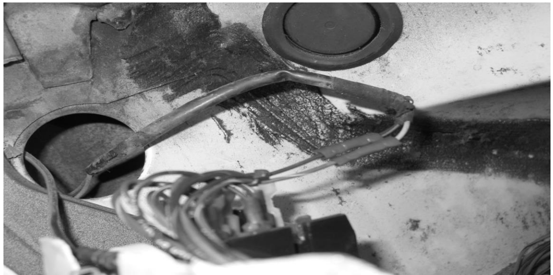
Figure 7-26 Door Jamb Switches – 1973-1977 Models
