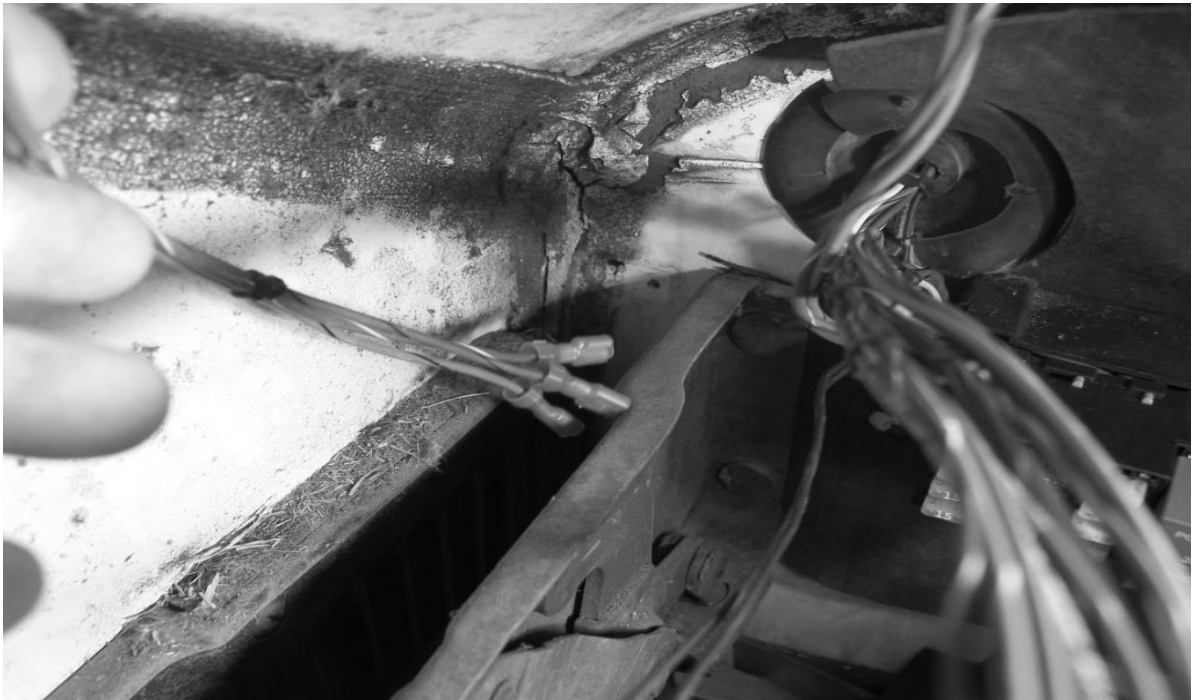
Figure 7-22 Routing the Dimmer Switch Wires
