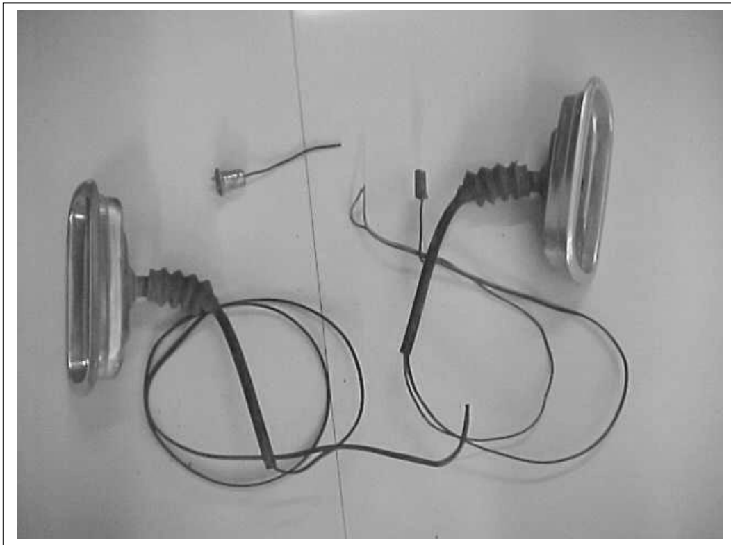
Figure 7.13 Tail Lights and License Light (after being removed)
