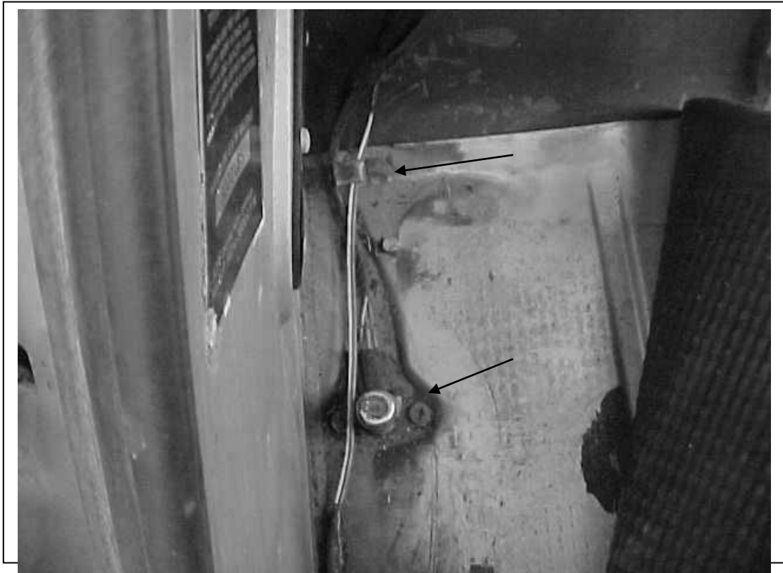
Figure 6.7 Routing of the Cab Section. Down from the fuse block and through the groove in the door jamb. Arrows are pointing at the Dimmer Switch and a mounting bracket.
