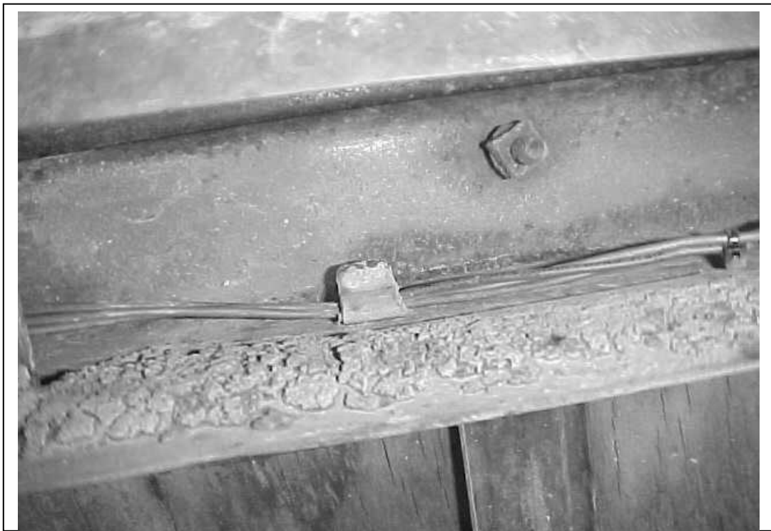
Figure 6.6 Mounting brackets are along the frame for your Tail Section mounting.
