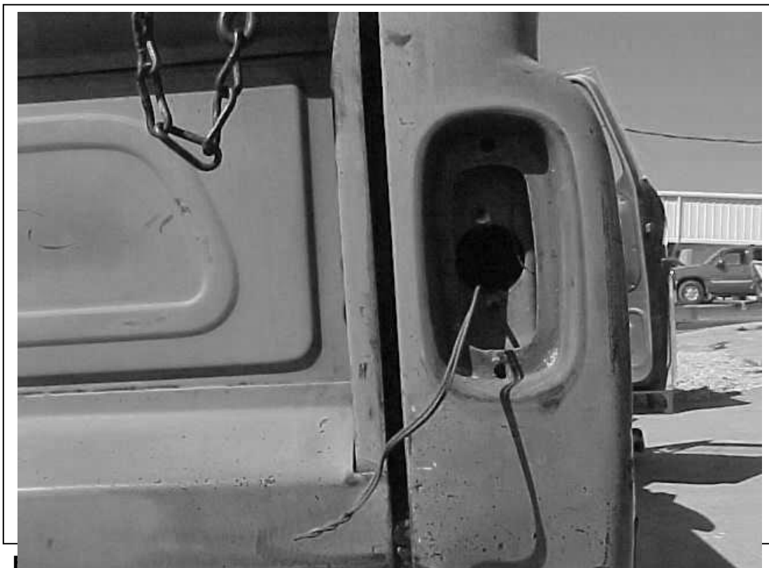
Figure 7.13 Tail Lights and License Light (after being removed)
